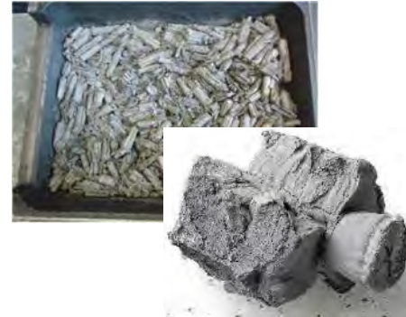
HM-Scrap after Zn-processing
